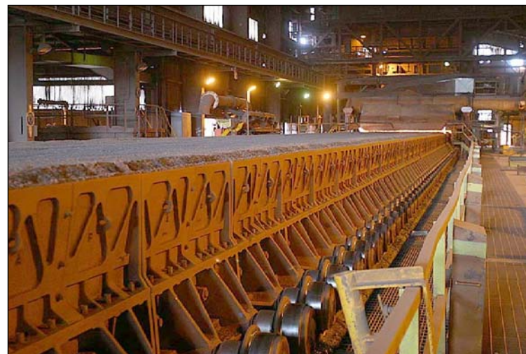
The strand within the Sinter Plant. The ignition hood is at the rear of the photo.
