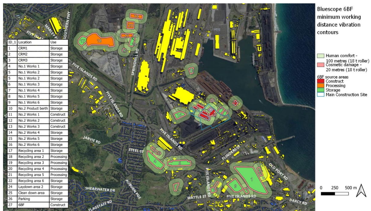
Figure 7 Minimum working distance contours (18 t vibratory roller)
