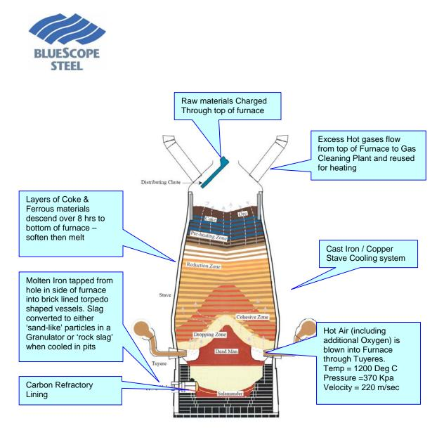
Figure 5 Process flow through No.5 Blast Furnace
